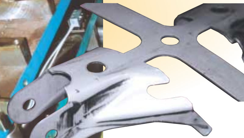
TT&D likes the flexibility offered by its programmable lubrication stations, so that its ability to lubricate dies doesn’t limit the type of job in can run. It won this job—upper-suspension control-arm brackets—in March 2002. Running the 12-station progressive die, lubrication is provided by a roller at the entry end complemented by four nozzles in the die—two at the form station and two more at the cam-pierce station.
